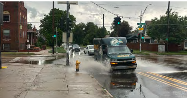
Figure 6 Corner catch basins and valley gutters can exacerbate ponding and snow accumulation, decreasing accessibility.
