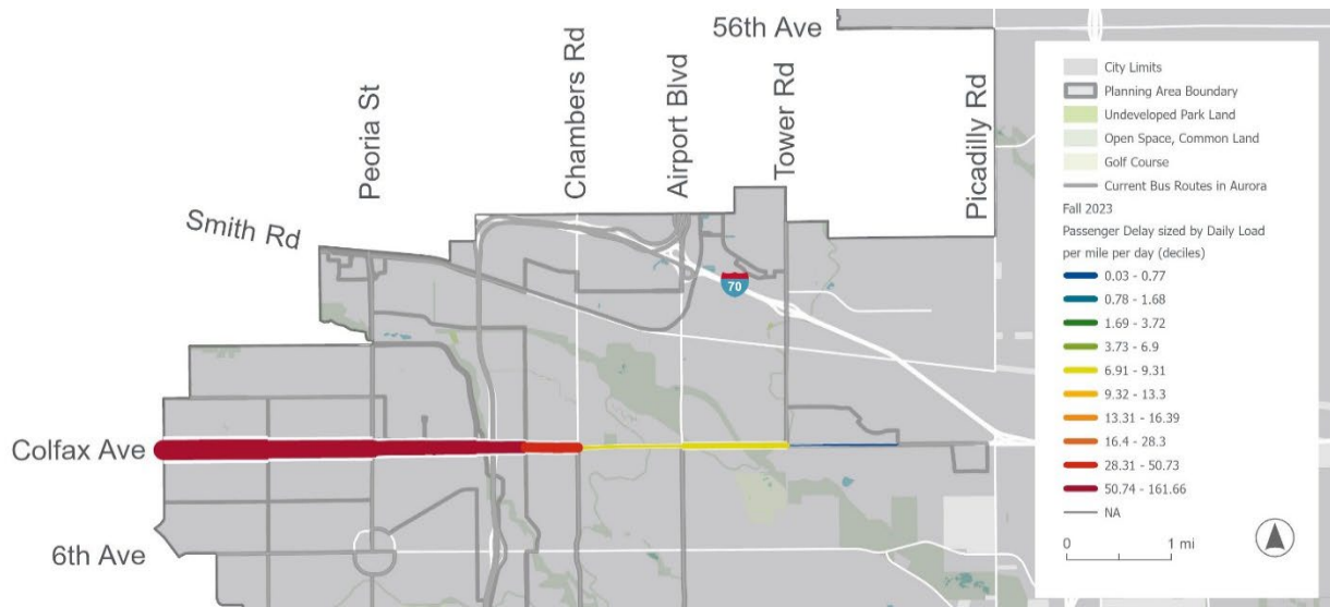
Figure 5-13: Colfax corridor passenger delay
